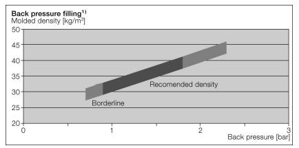
$^{\rm 1)}$  The Processing data are determined on molded parts (300 x 200 x 60 mm) produced under standard conditions and steam pressure of 3.2 - 3.6 bar. The data apply for average bulk densities.
