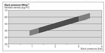
$<sup>^{1)}</sup>$  The Processing data are determined on molded parts (300 x 200 x 60 mm) produced under standard conditions and steam pressure of 3.2 - 3.6 bar. The data applies for average bulk densities.
