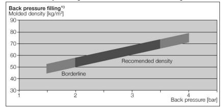
$^{1)}$  The Processing data are determined on molded parts (300 x 200 x 60 mm) produced under standard conditions and steam pressure of 3.2 - 3.6 bar. The data applies for average bulk densities.
