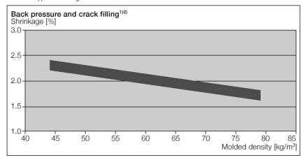
2) Shrinkage after oven curing (80 °C)
