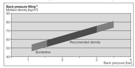
$<sup>^{\</sup>rm 1)}$  The Processing data are determined on molded parts (300 x 200 x 60 mm) produced under standard conditions and steam pressure of 3.2 - 3.6 bar. The data apply for average bulk densities.
