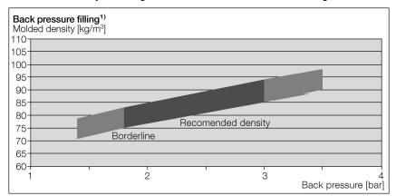
$<sup>^{1)}</sup>$  The Processing data are determined on molded parts (300 x 200 x 60 mm) produced under standard conditions and steam pressure of 3.2 - 3.6 bar. The data apply for average bulk densities.
