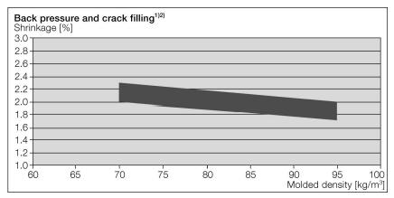
$<sup>^{2)}\,</sup>Shrinkage after oven curing (80 <math display="inline">^{\circ}C)$
